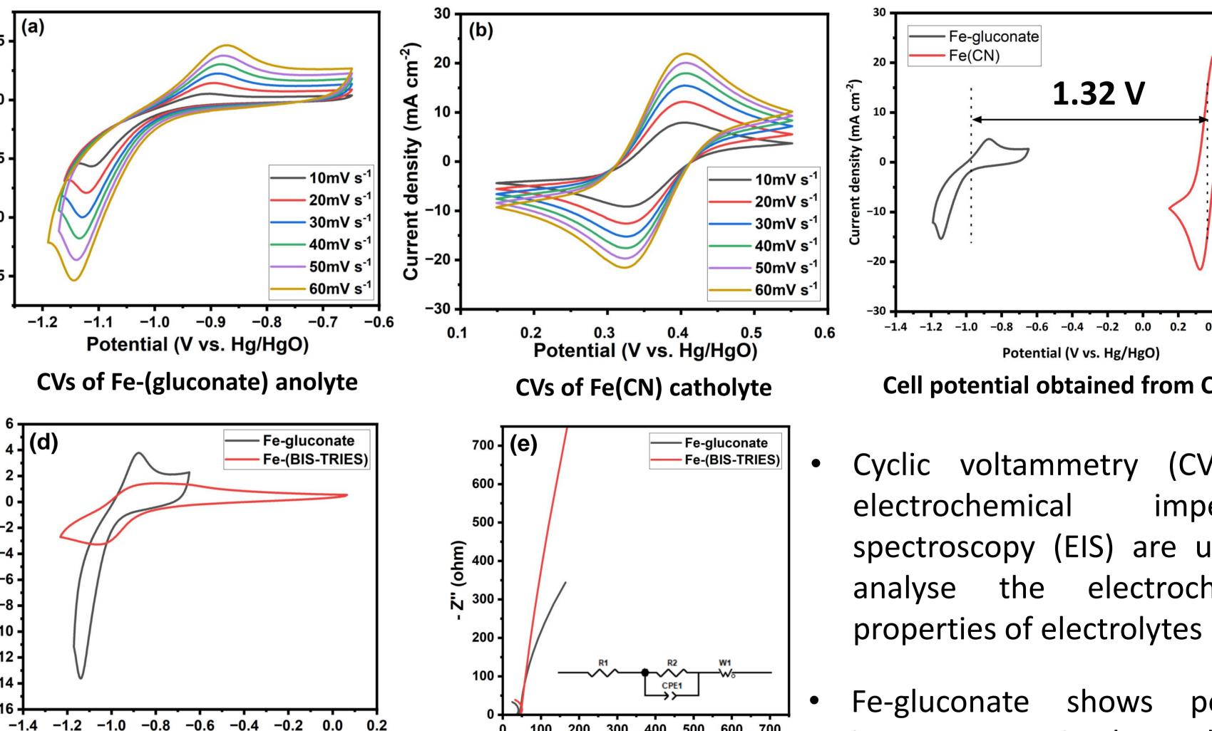
Potential (V vs. Hg/HgO) Cell potential obtained from CV test Cyclic voltammetry (CV) and electrochemical impedance spectroscopy (EIS) are used to the electrochemical
