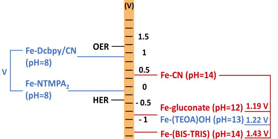
Fe-Gluconate Based Redox Flow Battery
